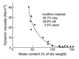
Fig. 4. Relation between viscosity and water content (after Bentley, 1979).
