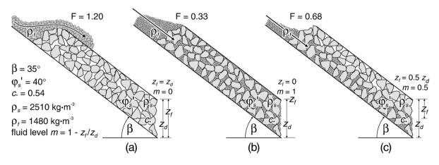
Fig. 5. Three typical situations if a rock-fluid mixture reaches an accumulation of coarse debris.
