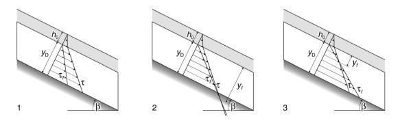
Fig. 2. Characteristic shear-strength and shear-stress distributions in saturated debris (after Takahashi, 1978, 1980).
